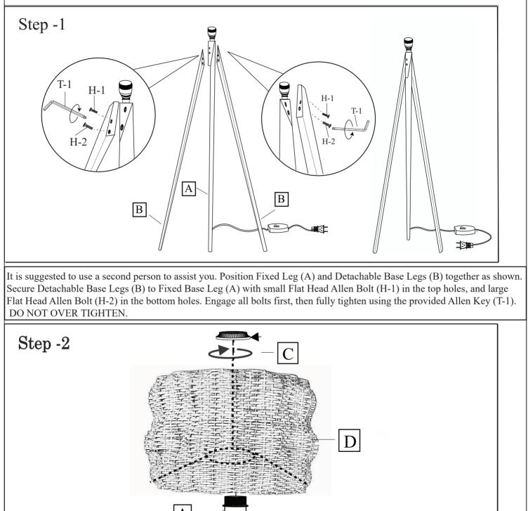
Remove Uno Ring (C) if it is pre-attached to light socket. Place Lamp Shade (D) onto the light socket on top of the assembly from Step 1. Secure by re-attaching Uno Ring (C) onto light socket. Tighten until snug. Remove any plastic wrapping on the Lamp Shade (D) before use.
