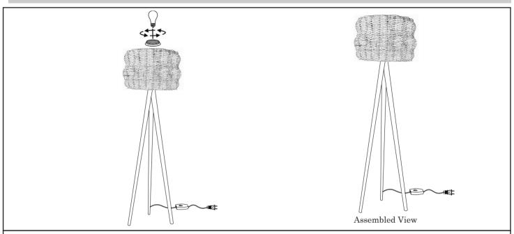
Insert Bulb (E; not included) into the light socket and rotate it clockwise to secure. Plug in lamp to a near socket and check for proper lighting operation. Assembly is not complete and the product is ready for use.
